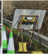
The CCT can also be deployed as an emergency call point for road users to summon vehicle recovery services. Having an accident or breakdown in the middle of road works can be a worrying time so having a readily accessible emergency call point provides vital comfort and reassurance to road users. At the push of a button, they can speak with someone, explain their emergency situation and get reassurance that help is on its way.
